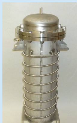
sorption reactor with cooling coil
