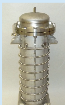
sorption reactor with cooling coil
